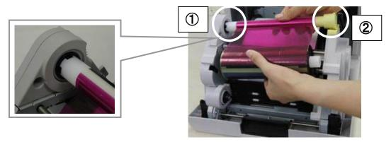
8. Set the supply side of the ribbon to the printer carefully to take out any slack. Insert the protrusion of the core left side in the hole on the printer, then set the right side to the holder of the same color (white). Take up the ribbon slack by rotating the ribbon on the supply side.
