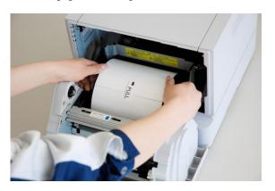
4. Remove a paper fixed tape, and Insert the paper.
