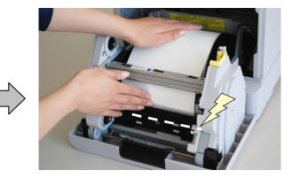
7. Set the take-up side core of the ribbon to the printer. Insert the protrusion of the core left side in the hole on the printer, then set the right side to the holder of the same color (yellow).
